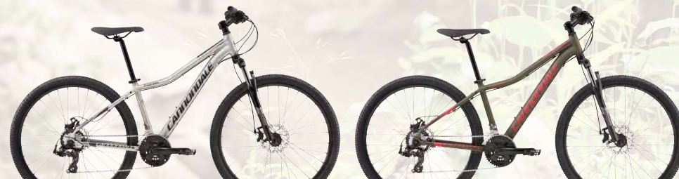
FORAY 4 FRAME Foray, butted 6061 alloy FORK SR Suntour M3030, 75mm, coil RD/SHIFT/CRANK Shimano Tourney-EF41 Easyfire / Prowheel, 24/34/42 BRAKES jak-7 cable disc WHEELSET Alex DC 6.0 - 27.5" COOL BITS Cannondale C-Series cockpit / Stage 2 Women's Saddle COLOR Fine Silver w/ Nearly Black, Charcoal Grey - Gloss (SLV) / Green Clay w/ Magenta, Mulberry - Matte (CCL)
